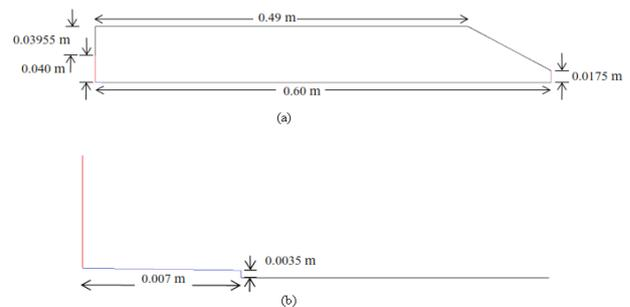
Figure 2. Dimensions of mini spray dryer (b) Dimensions of feed inlet
