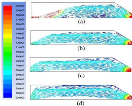
Figure 7. Effect of initial particle size under Set 1 operating condition at (a) 36  $\mu\text{m}$  (b) 79  $\mu\text{m}$  (c) 123  $\mu\text{m}$  (d) 123  $\mu\text{m}$
