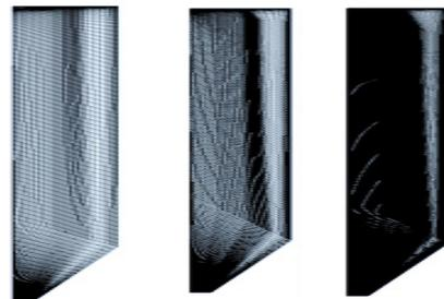
Figure 3. Geometry of spray dryer (a) 0.015 mesh size (b) 0.01 mesh size (c) 0.005 mesh size
